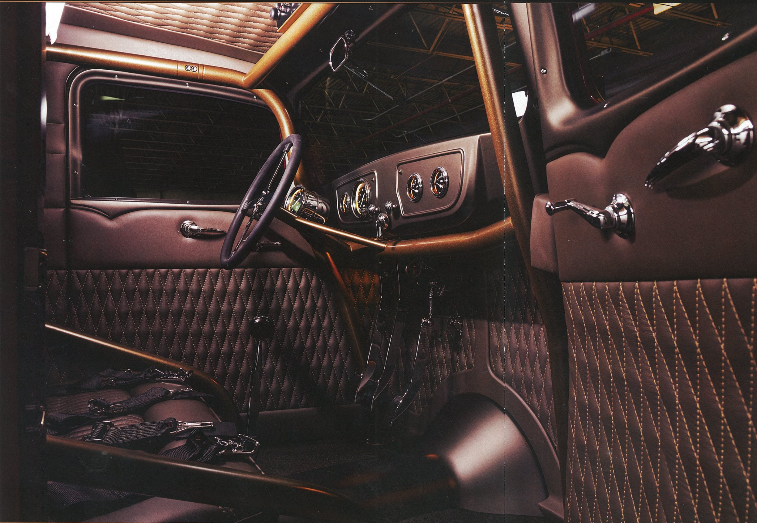
Schober's Custom Hot Rod Interiors laid out a beautiful cabin that pays tribute to the original but is finished out to show car quality. The reworked stock dash houses Classic Instruments gauges and one-off knobs for the turn signals and wipers. The overhead switch panel looks vintage but is a custom machined piece. Datum Tool and Manufacturing performed the CNC work.
