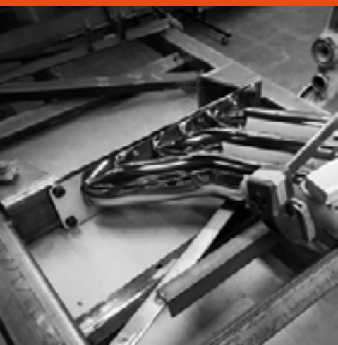
After all the tubes were polished they were fit back in the welding fixture and final welded.
