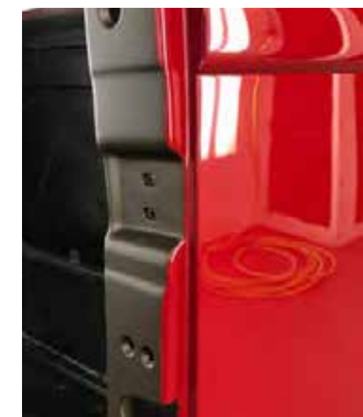
After the body and doors were color sanded and polished, the interior of the truck cab and the jambs were painted with Audi Marrom Bronze that matches the drivetrain color.
