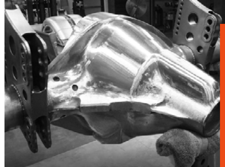
This photo was taken during the first stage of smoothing the rear end housing casting with 50 grit. We took the rear end to 120 grit sanding everything smooth and blending it so it looked like glass before handing it off to the body shop for paint.
