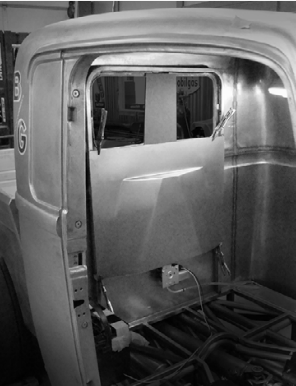
Completed roll down rear glass assembly with power window regulator cover being located and mounted.
