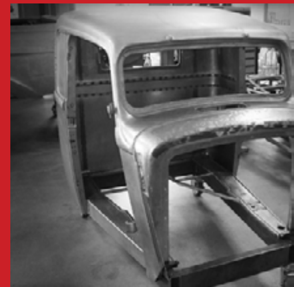
Finishing weld seam across the top of the cowl with the cab off to gain more accessibility for hammer and dolly work.
