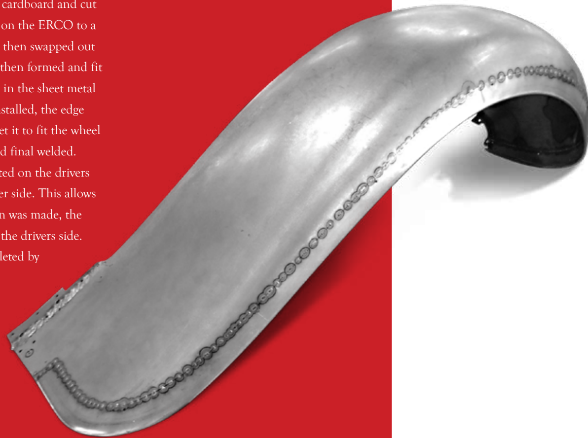
Final fit and locating the symmetrical wheel opening on the front fenders took some patience to get it right.
