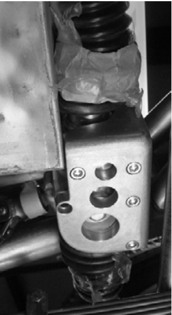
There was fortunately just enough room to squeeze the rack & pinion in front of the oil pan.
