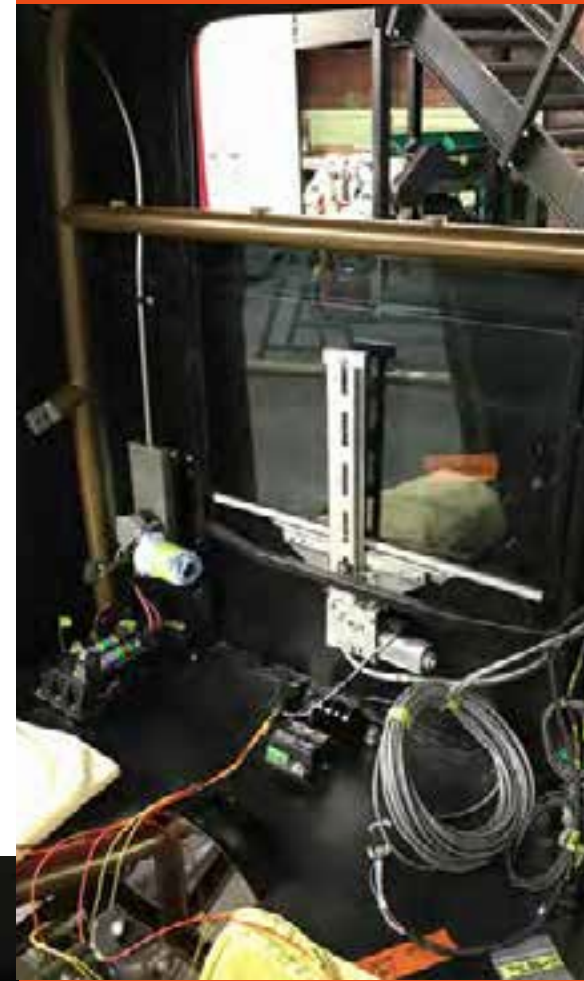
Everything has a place and it's in its place. Wiring all hidden under the bench seat, batteries, fuse panels, computers, relays etc. all engineered to fit so nothing is mounted under the dash.
