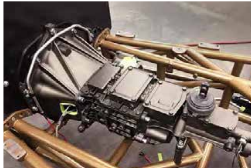
Tremec TKO 5-speed transmission installation
