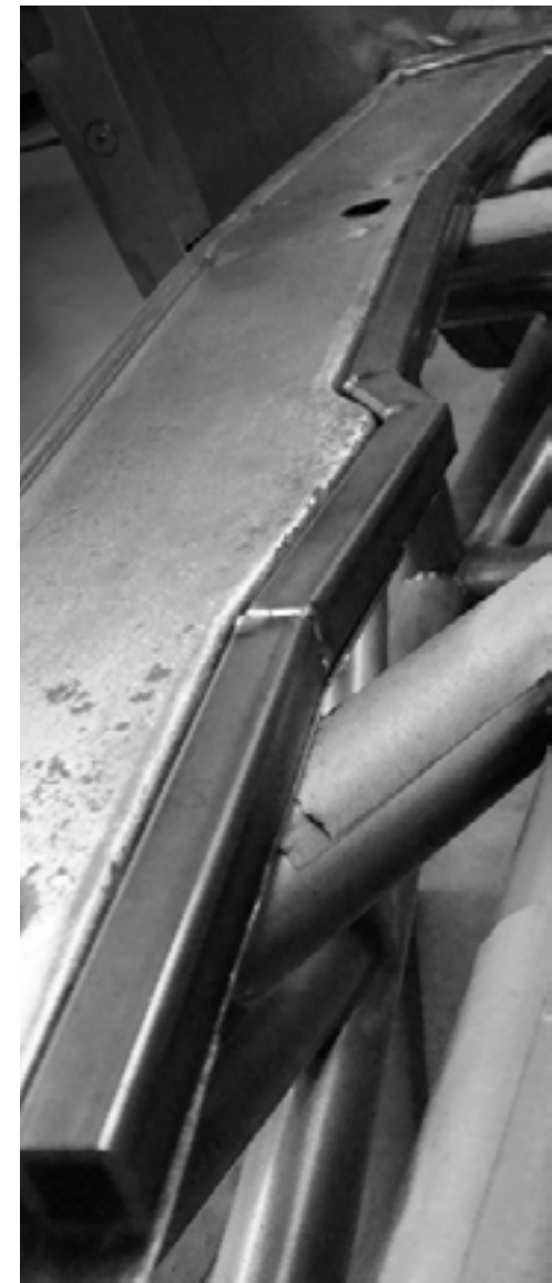
Steel tubing was used to fill the void of the original plywood floor. The new removable sheet metal floor was bolted to this framework.
