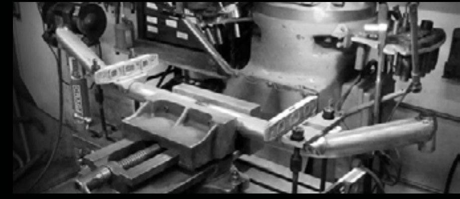
Utilizing the Bridgeport vise to locate and then tack weld the axle mounting pads to the axle.
