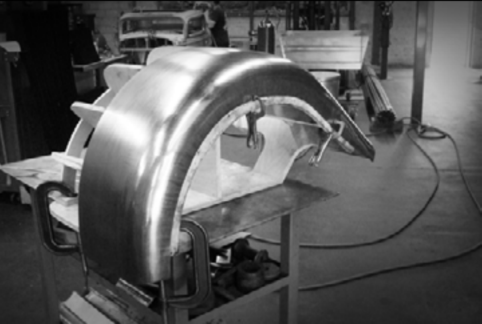
The final shaped rear fender made from one piece of 19 gauge steel clamped to the buck.
