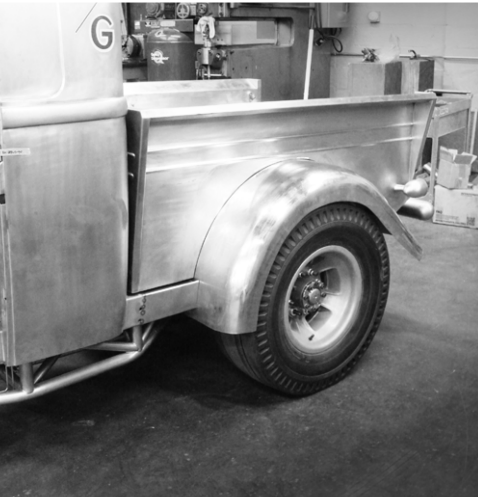
Extending the original rocker to make it line up with the new fender location and wheel base.
