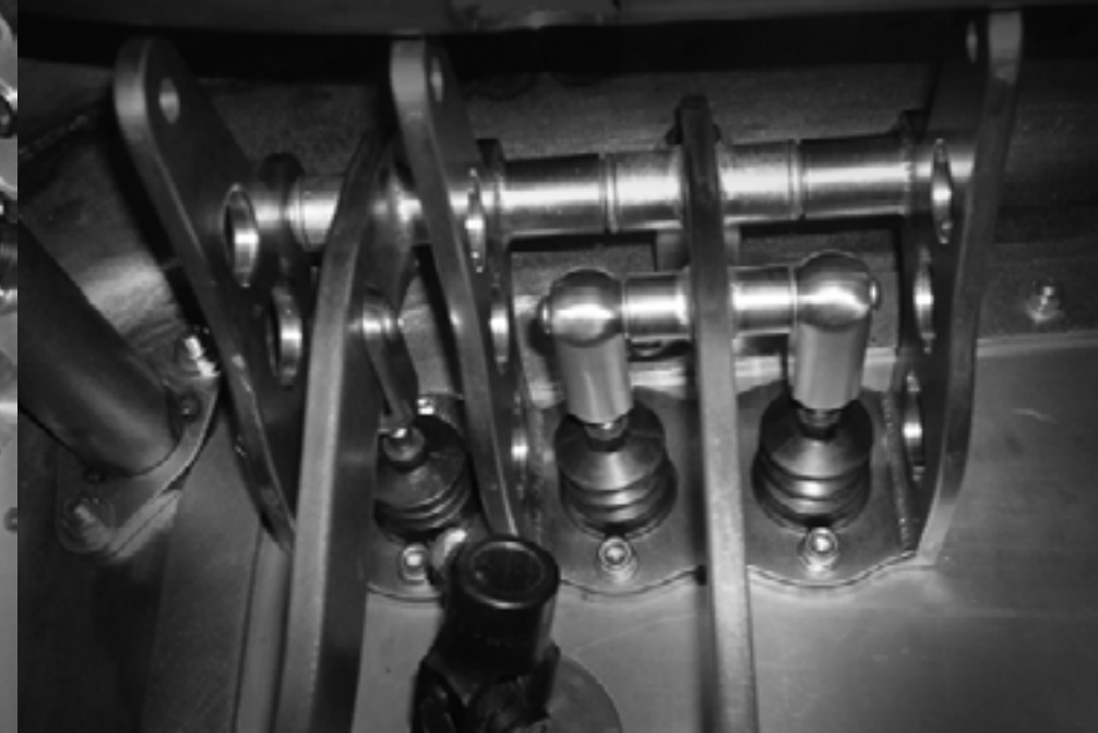
One-off fabricated and machined components make up the entire brake and clutch pedal assembly.
