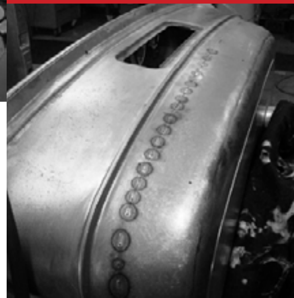
Finishing weld seam across the top of the cowl with the cab off to gain more accessibility for hammer and dolly work.
