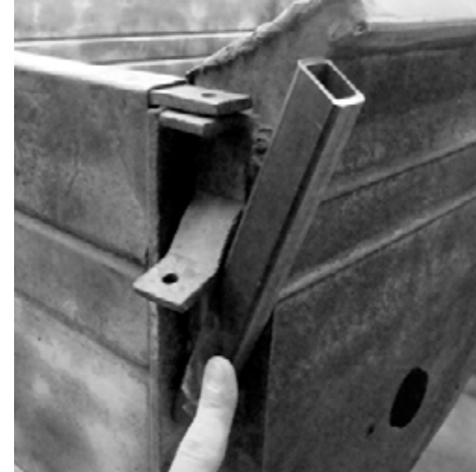
Mapping out some general design concepts with 1" square tubing to create a stake pocket design.
