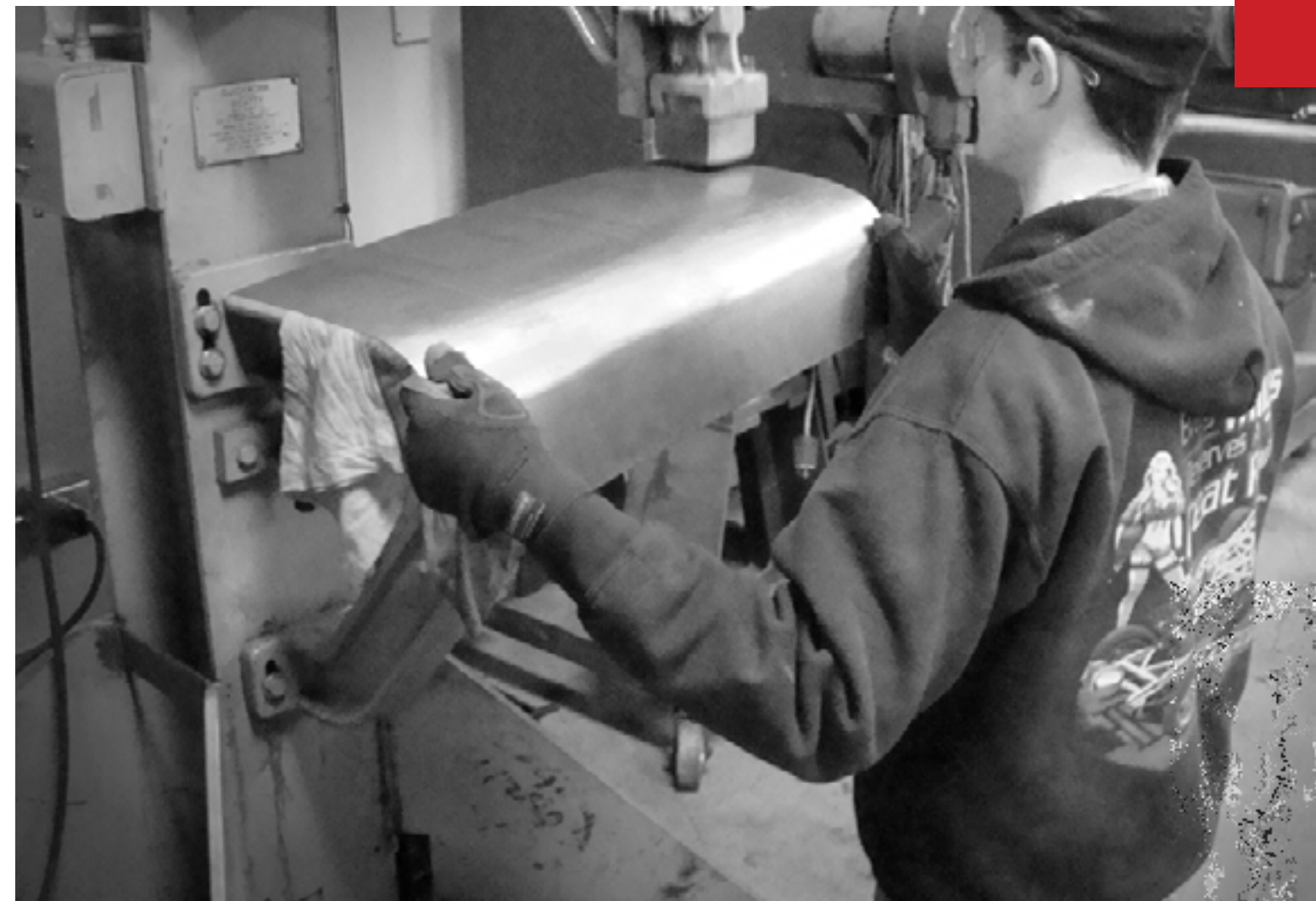
Shaping the lower section of the cab in three separate pieces: The sides were both shaped and fit to the buck and then the center was shaped.
