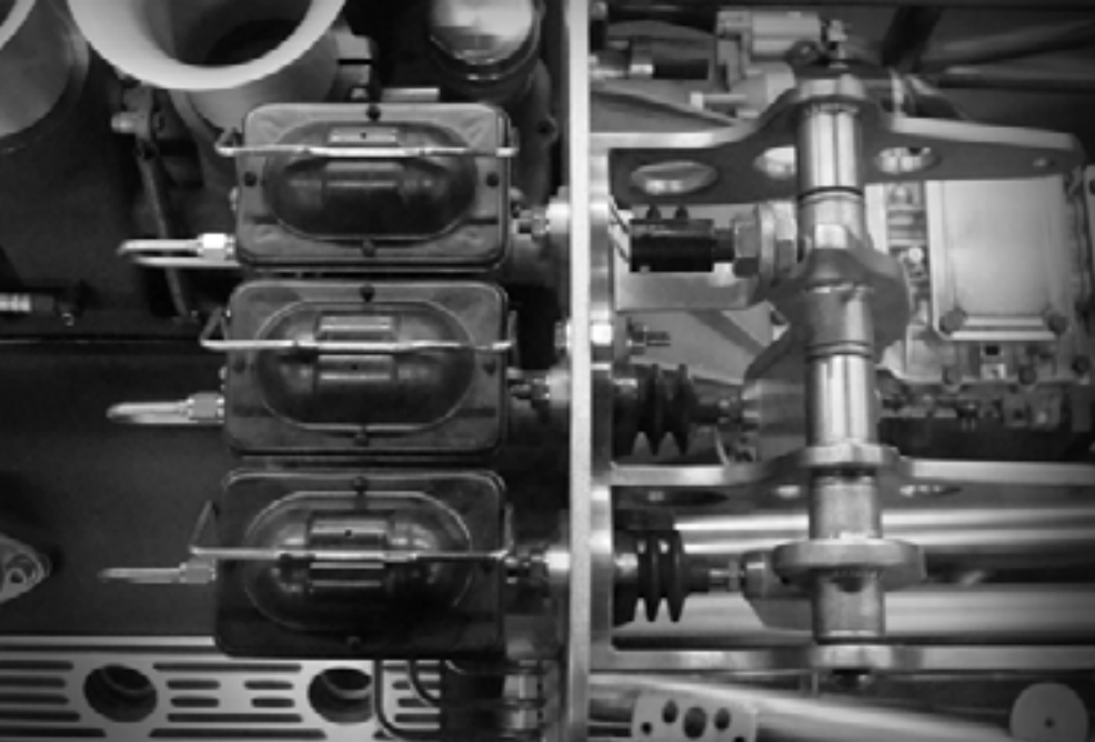
Master cylinders and pedal assembly from a bird's eye view.
