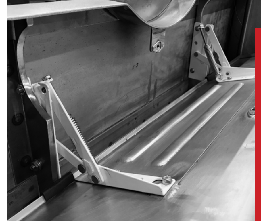
Spring-assisted hinges for front hatch close-in panel hold panel when open and help adding closing assistance.
