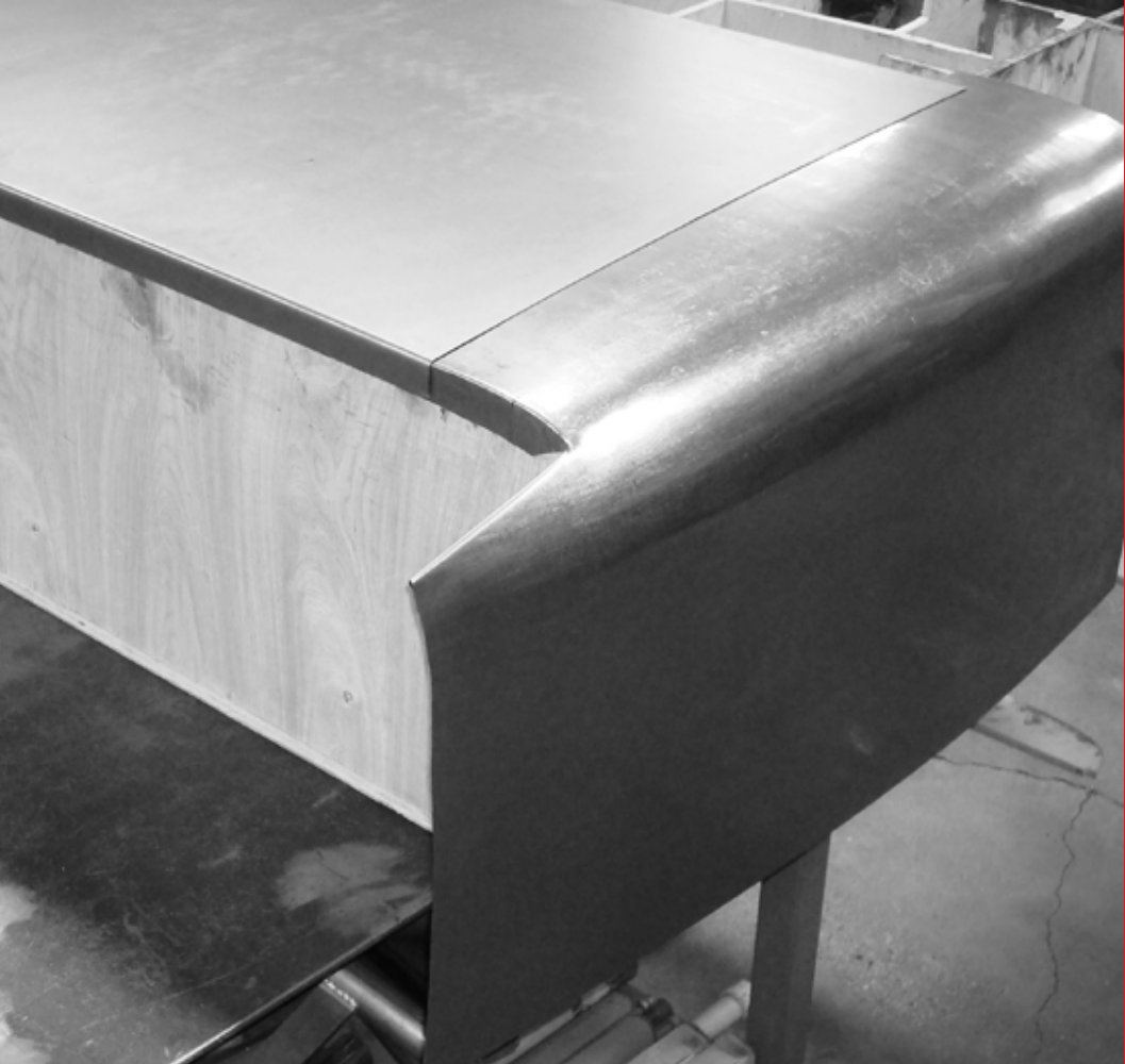
I believe the back of this truck cab gets the award for the lowest crown panel we have ever shaped.
