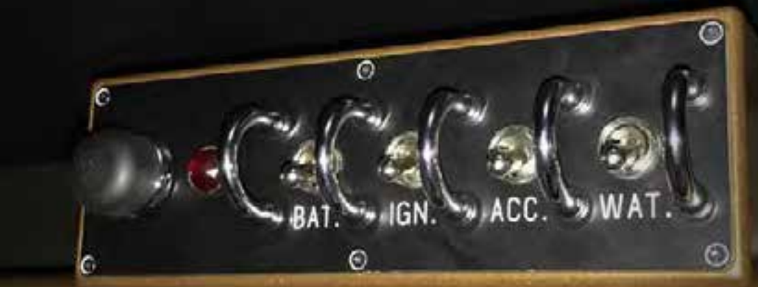
Shot of overhead switch panel final installation. Engraved typeface matches gauge typeface, vintage red jewel for ignition matches green vintage turn signal indicators in dash. Chrome plated push button starter bezel and finger guards.
