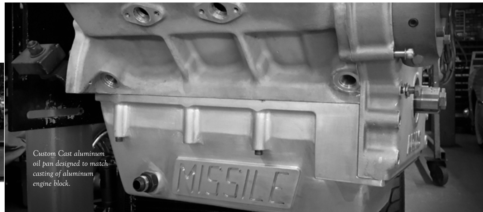
Machined side block water manifolds were shot peened to resemble the cast look of the rest of the engine
