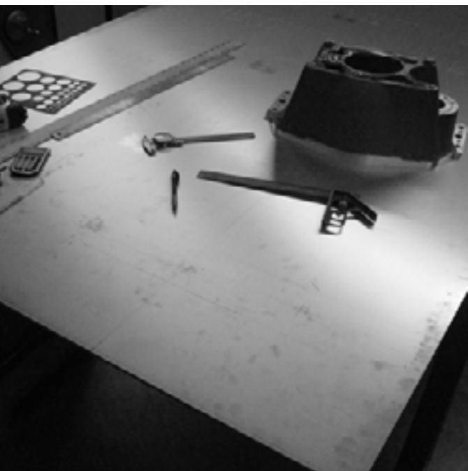
Laying out mid-plate mounting holes to the frame and engine dowel pins for bell-housing.
