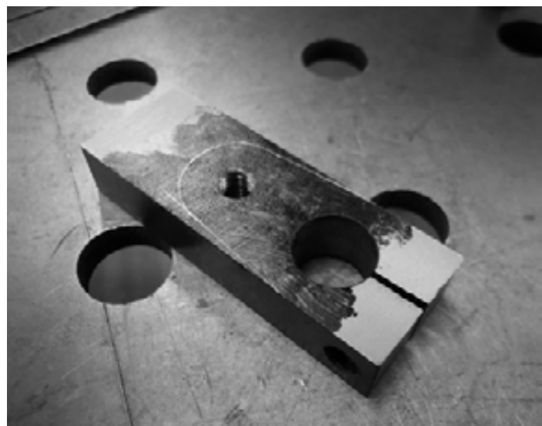
Detail of the throttle pedal bell-crank during the machining and fabricating process.
