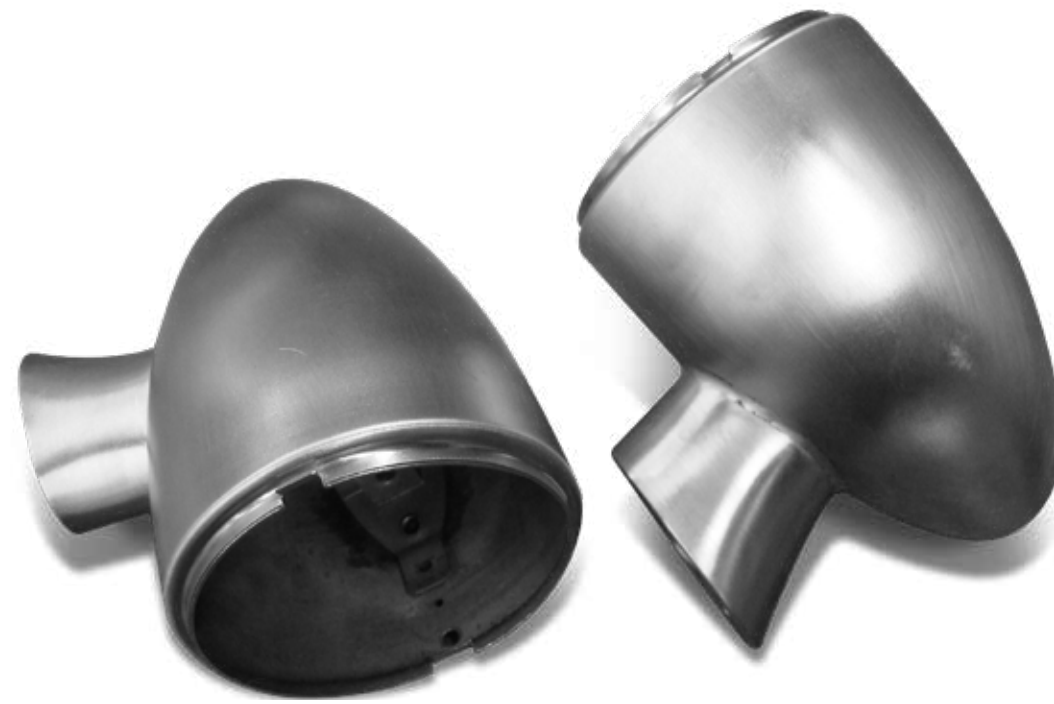
Designing and fabricating an elegant stand off for a pair of '37 Ford taillights. We also installed a piece of tubing to route the wiring through so there would be no exposed wiring on the backside of the bed.
