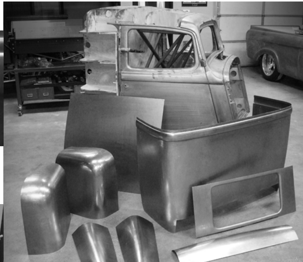
Finished panels ready for more fitting and welding to make sub assemblies.
