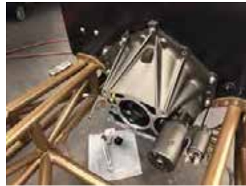
Clutch and bell housing installation
