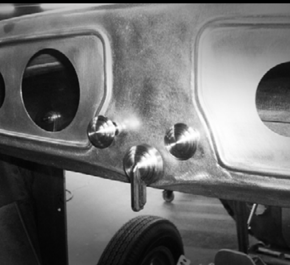
Finished knobs machined from 304 stainless steel.
