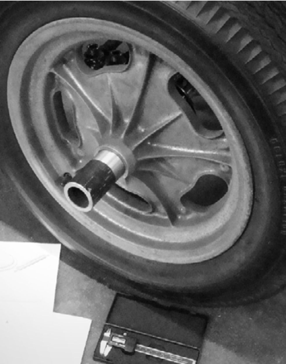
Mock up tool to test o-ring size to hold on cap when designing spindle caps for machine shop.
