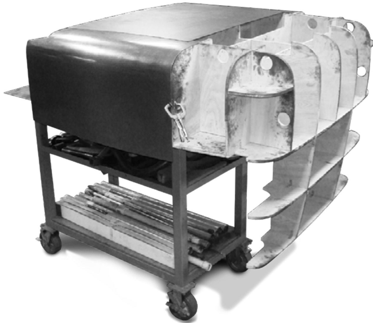
Shaping the lower section of the cab in three separate pieces: The sides were both shaped and fit to the buck and then the center was shaped.
