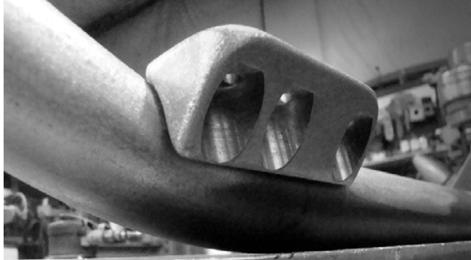
Spring perch counter-bored holes for axle u-bolts and sway bar/shock mounting bracket.
