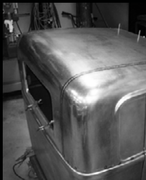
There was a lot of time spent welding and metal finishing the major seams before the entire assembly was permanently affixed.
