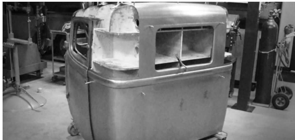
Finished panels ready for more fitting and welding to make sub assemblies.
