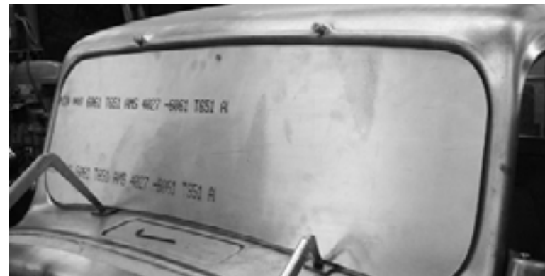
Locating the template for the flush-mount windshield so we didn't have to use the ill-fitting OEM style rubber.
