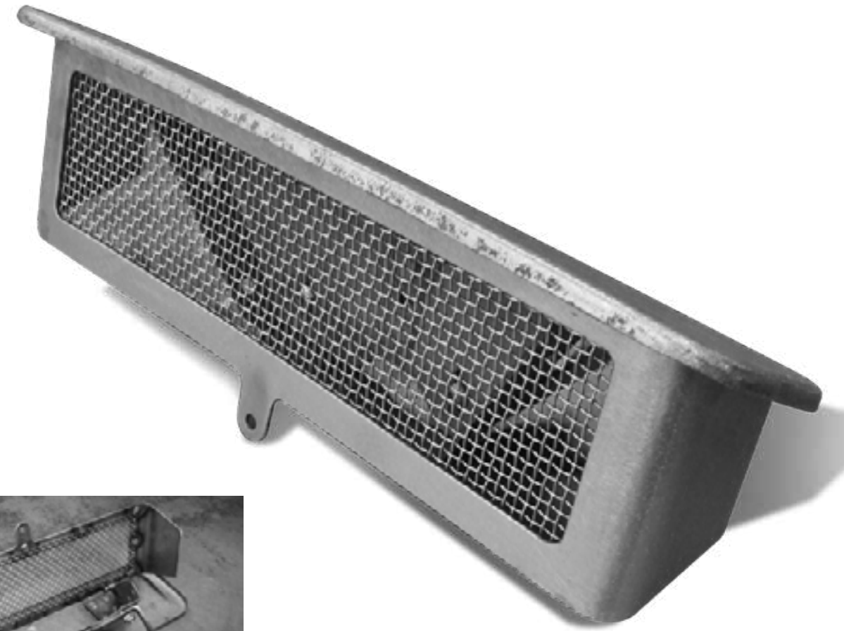
After the major modifications to the hinging insert with rollers a simple stainless screen was permanently welded to the insert from the backside.
