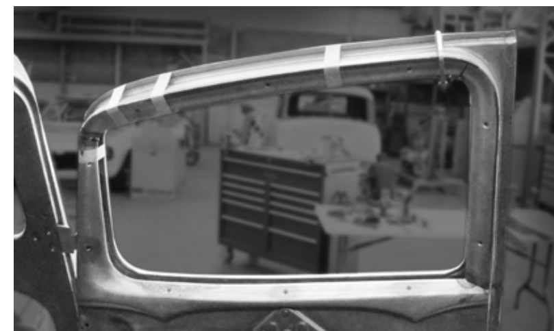
Reworking the garnish molding so they fit the door top better and the edges were more flush.
