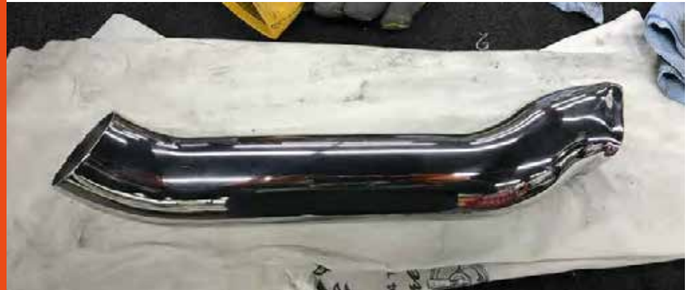
Fully polished 2 1/2" diameter 304 Stainless steel zoomies.
