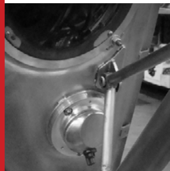
We utilized axle caps from a utility trailer and hammering flat spots to clear the grille shell supports. We mounted the light socket in the lower half.
