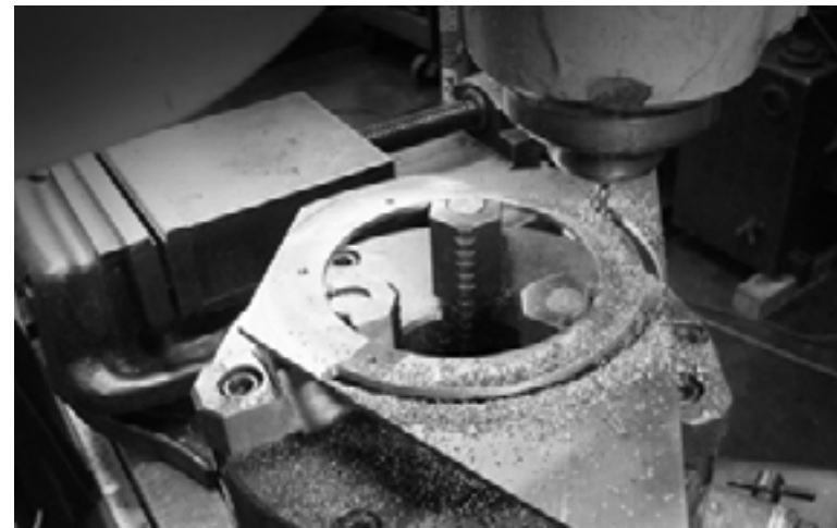
Machining the shifter handle and the boot bezel from scratch.
