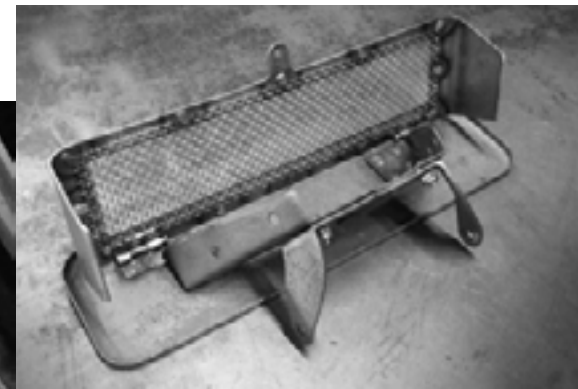
After the major modifications to the hinging insert with rollers a simple stainless screen was permanently welded to the insert from the backside.
