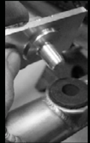
Detail of flush mount rubber insert under radiator tank incorporated into the front frame cross member.
