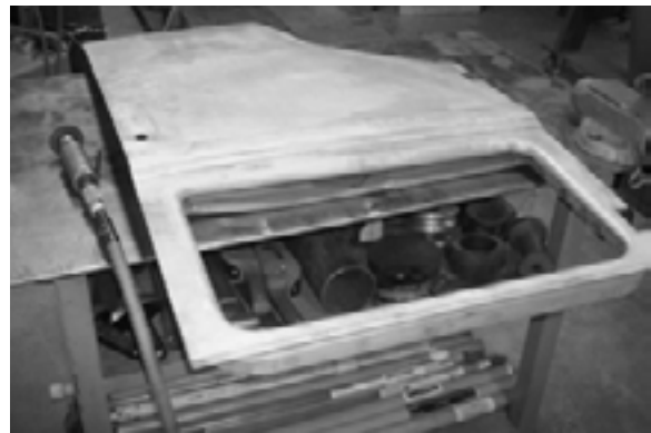
Cannibalizing a '36 Willys Rear Door for the trucks back window. Utilizing this OEM sheet metal with the roll up window run channels allowed us to make the back window roll up and down like a door typically would.
