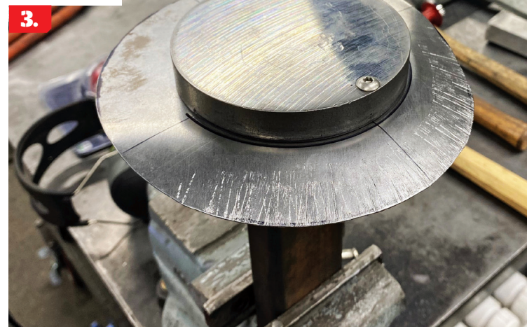
5. The metal is hammered down against the form while it's red hot.
