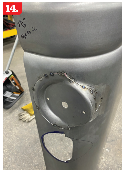
13. After the opening is trimmed to size, a hammer and T-dolly flare out the metal to fit the mounting flanges.
