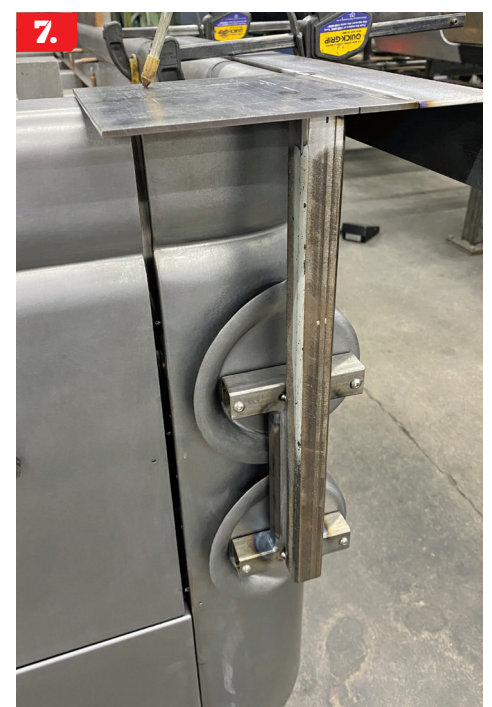
7. A sturdy fixture holds the hand-shaped mounting surfaces for each light and positions them accurately from the top and side of the bed.
