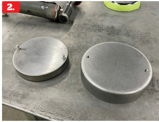
2. Hammerforms were made from steel plate to help form the mounting surfaces for each taillight assembly. Note that these are different-sized discs. 3. Here a disc of sheetmetal is clamped to the hammerform, and a metal shrinking machine is used to start moving one flange down on the shallower side of the recess.
