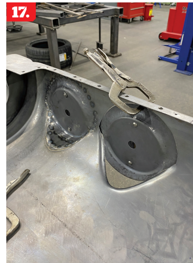
17. From the inside, you can see how well the edges are aligned.
