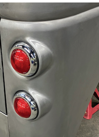
21. Here, the taillights are mounted on the passenger side. They look like they were designed for this application.
