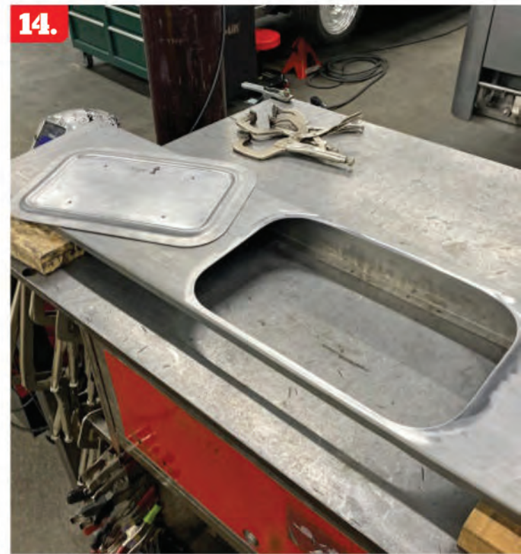
12. This is the finished piece after running the panel through the dies repeatedly, working incrementally toward full depth. You can see the fit against the license frame is spot-on.
