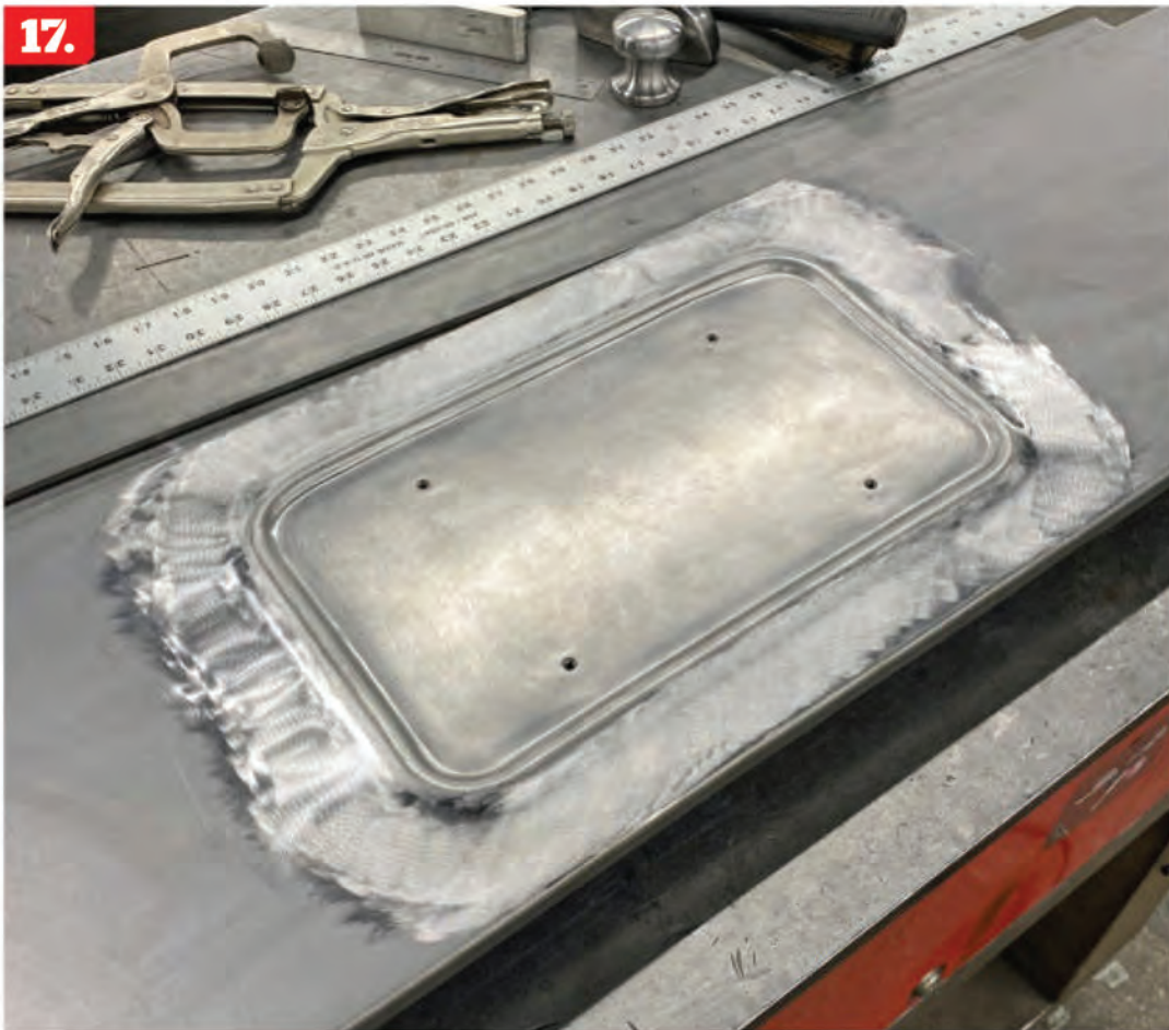
17. After welding and hammering, the welding bead is sanded flush.
