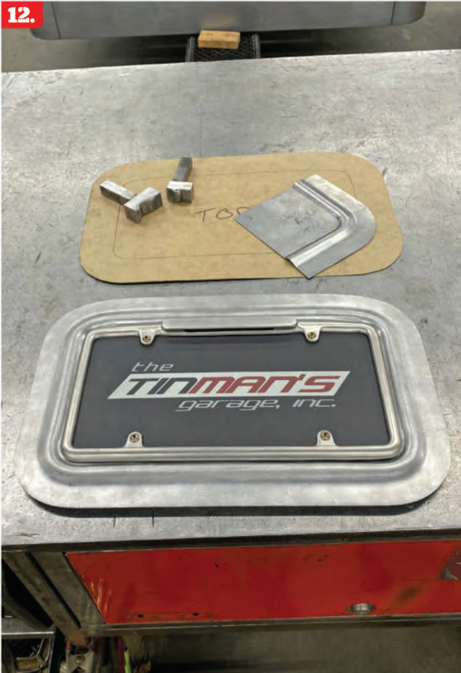
12. This is the finished piece after running the panel through the dies repeatedly, working incrementally toward full depth. You can see the fit against the license frame is spot-on.
